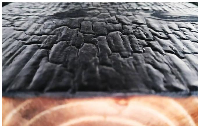
weather conditions as well as the type of wood that determines the adhesion of the charred layer. If you want to strengthen the charred layer, follow general care, wait 2-3 days for the wood to dry than using a roller, apply a coat of colorless acrylic paint intended for outdoor use.
