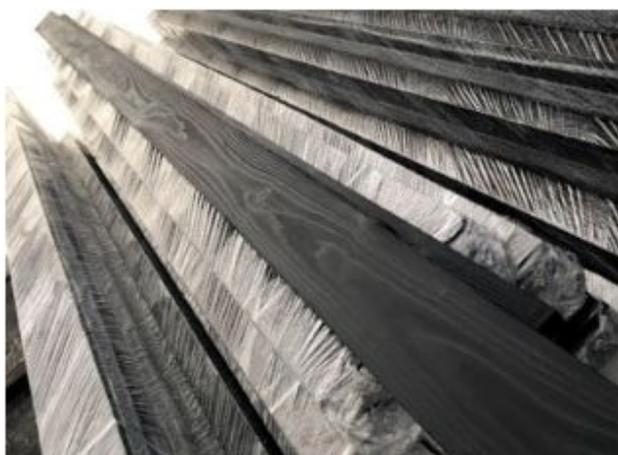
The moisture level of timber when painting must be below 20%, temperature at least +5°C and relative air humidity below 80%. Avoid painting in direct sunlight, since otherwise drying is too intensive and as a result the paint coating is less durable.
